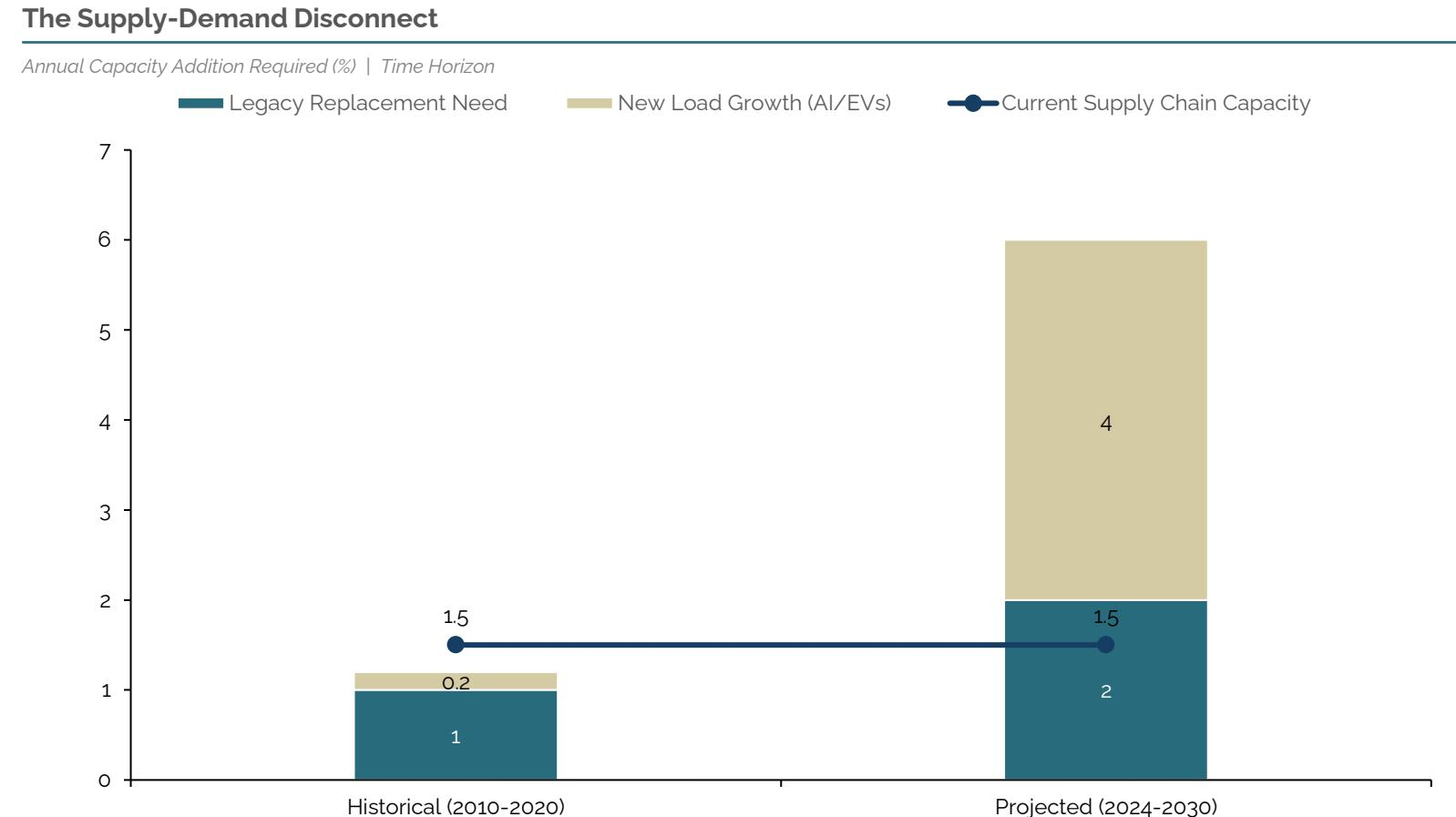
The specific nature of AI data center demand exacerbates the shortage, as higher power density racks require 3x the transformer capacity per square foot.
